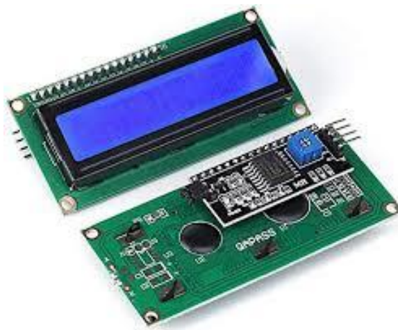
Figure 21 : Ecran LCD 16x2 i2C
