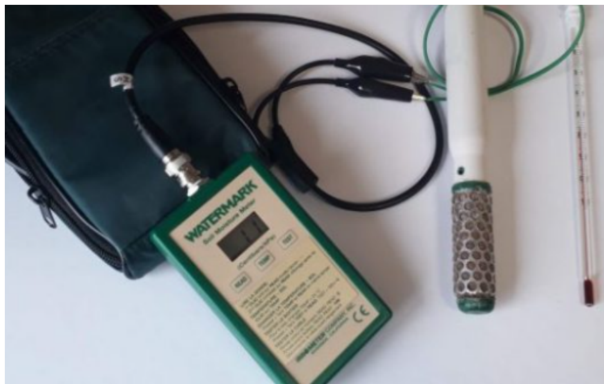
FIGURE II.8 – Kit de WATERMARK
