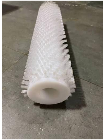
Figure 33: Nylon 6.6 brush bristle detail (component photo)
