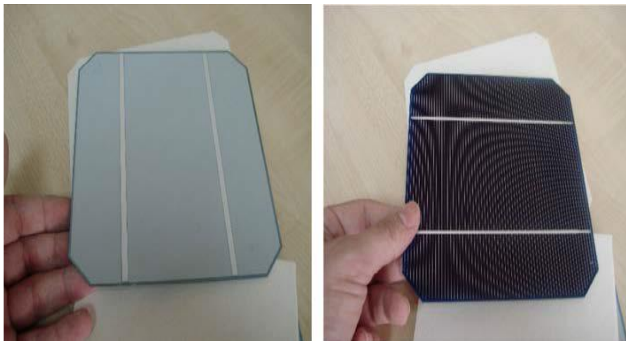
Fig. II.3: View from both sides of monocrystalline solar cells [112].
