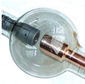
Figure II.4: Tube de Coolidge
