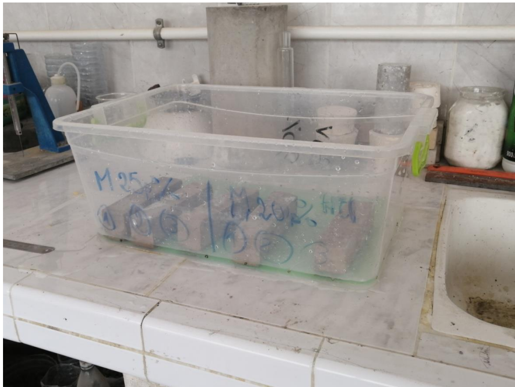
Fig.II.23. Principle of the capillary absorption test
