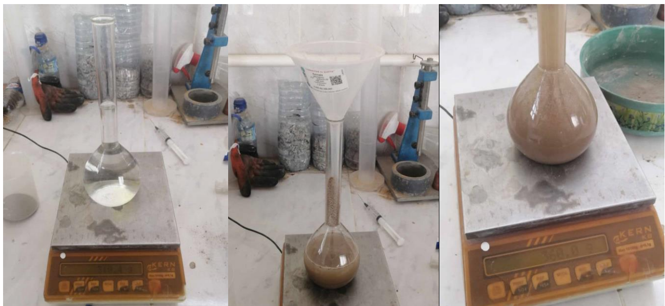
FigII.12. Operating procedure – Absolute density
