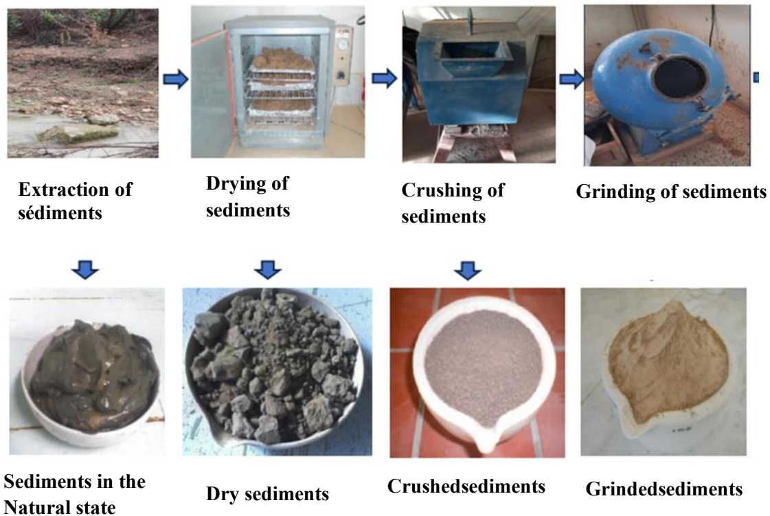
Fig.II.2. The processing stages of dredged sediments (Acchour, 2024).
