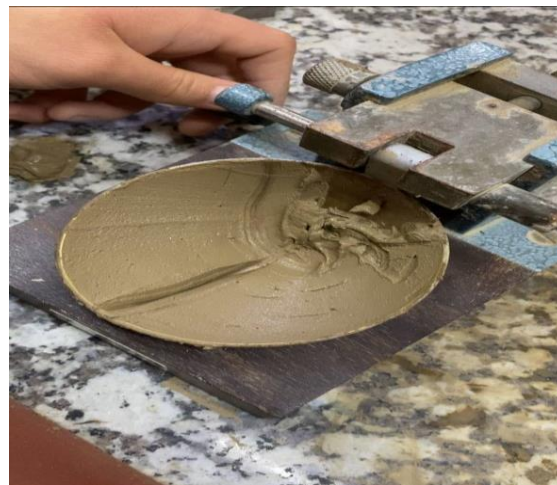
Fig.II.8. Contact between the two lips of the groove
