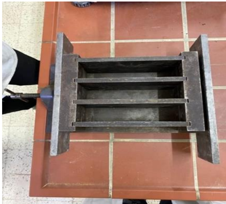
Fig.II.16. Mould used for manufacturing DSB
