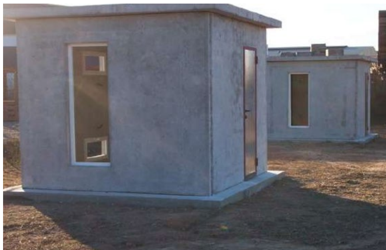
Figure 3.13. Experimental cabin (dimensions: 2.4 m × 2.4 m × 2.4 m)[94].
