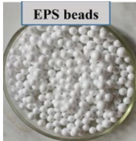
Figure. 2.3. Expanded polystyrene beads used to make clay bricks [36].
