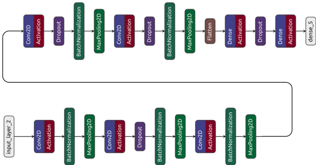
Figure 3.3: Pneumonia Detection Model Architecture
