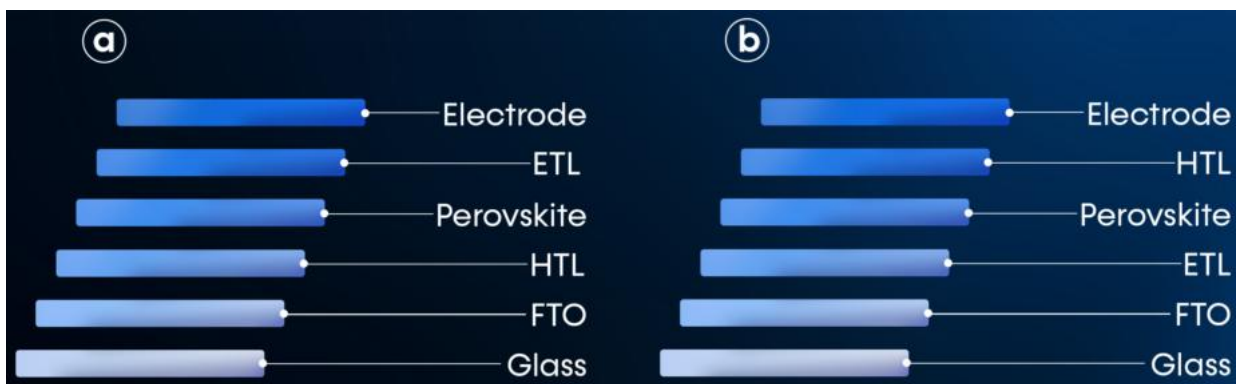
Figure VII.4. Diagram illustrates both n-i-p and p-i-n structures
