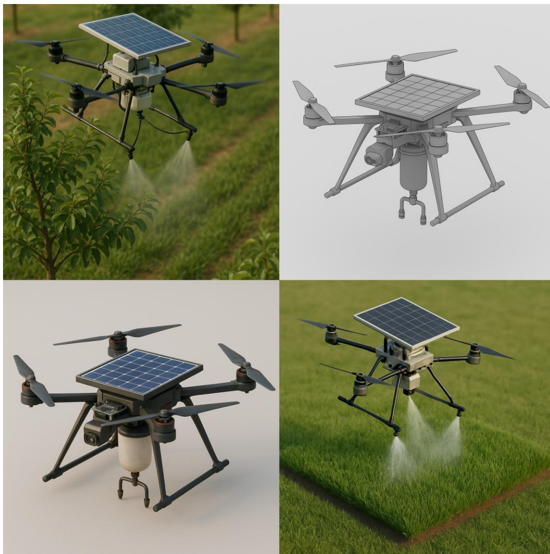
Figure VII.8. 3D View of Simulated Agricultural Quadcopter with Integrated Solar Panel
