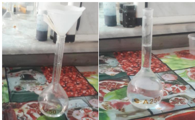
Figure III.2: Filtration de la saumure
