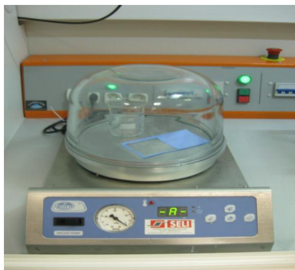
Figure III-8: L'étuvage des bandes LTCC
