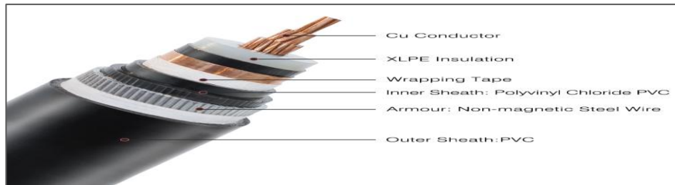
Figure II.13: Constitution d'un câble MT
