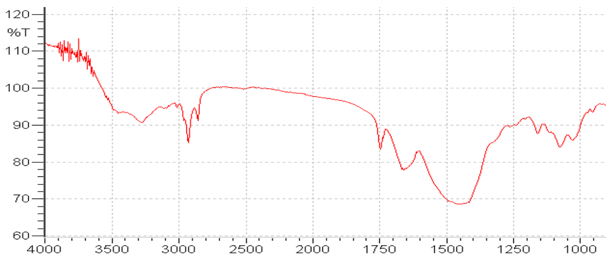
Figure 7 : Spectre Infrarouge de la chitine
