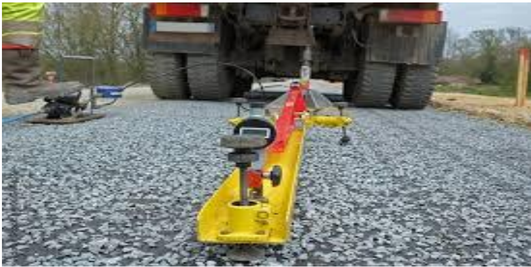
Figure II.8 : L'essai de plaque
