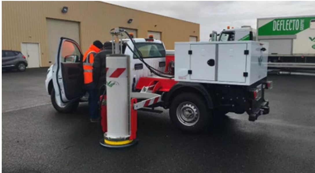
Figure II.16: Appareil Dyn plaque
