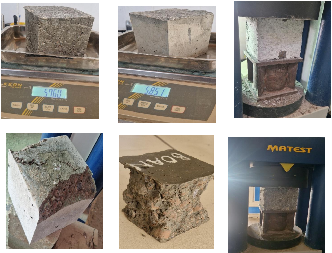
Figure II. 20 : Essai de compression.
