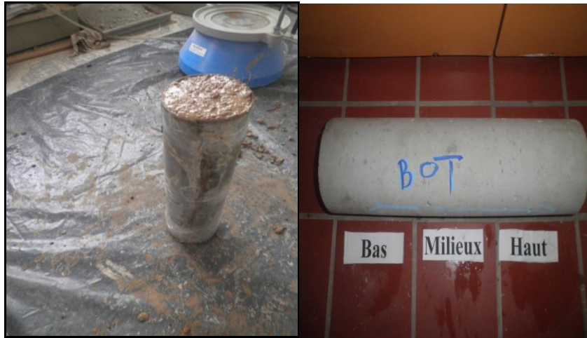
Figure II.14 : Essai de la colonne
