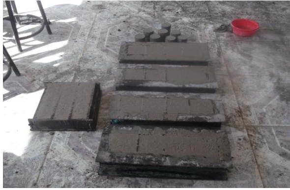
Figure II.16 : Coulage des moules (10x10x10) cm 3
