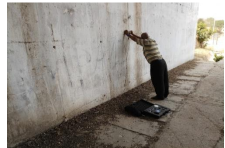
Figure 18: Essai ultrasonique de surface (transmission indirecte)
