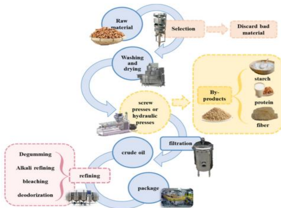
Figure 8: The preparation of tiger nut oil in food industry and by-products (Yali Yu et al., 2022).
