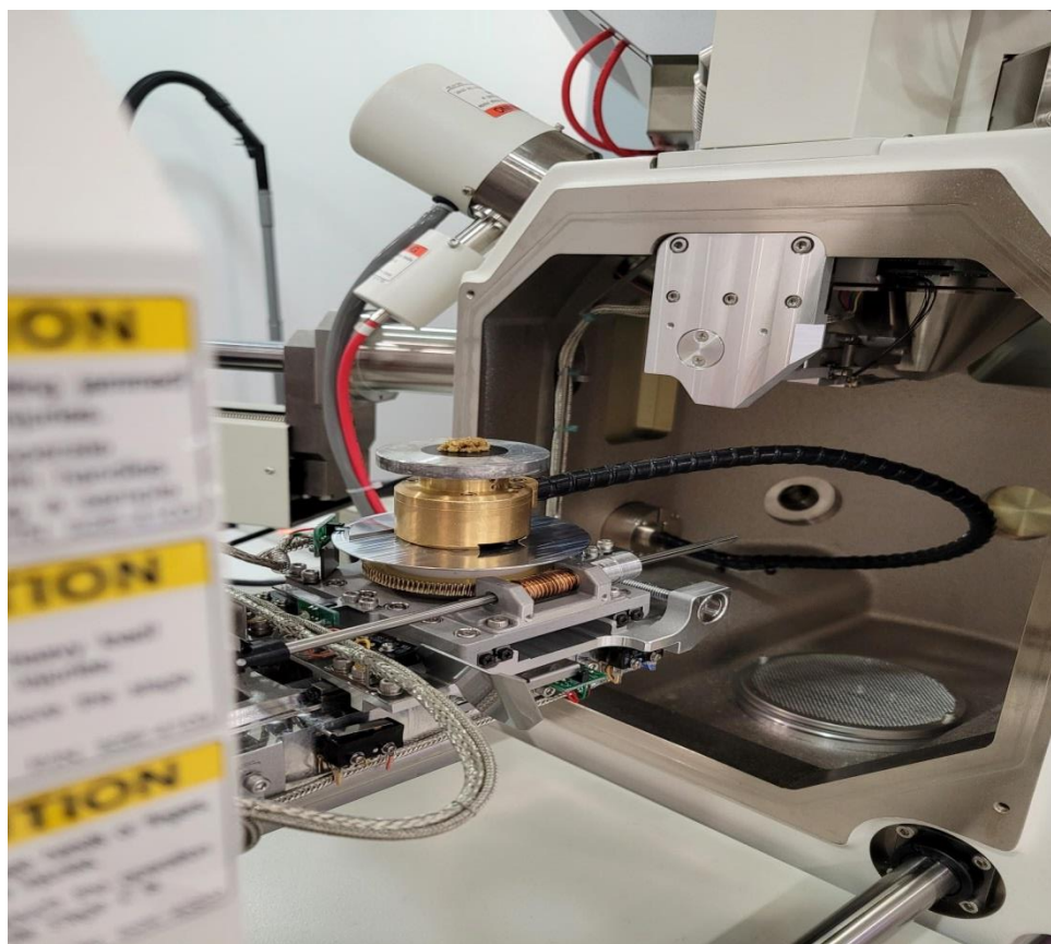
Figure 26: Scanning electron microscopy (FEG-SEM-LV SU-5000, Hitachi, Milexia, 91190-Saint-Aubin, France).
