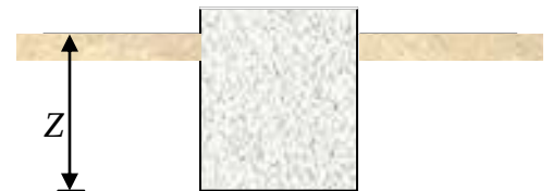
Fig.VIII .8: Encrage de la structure
