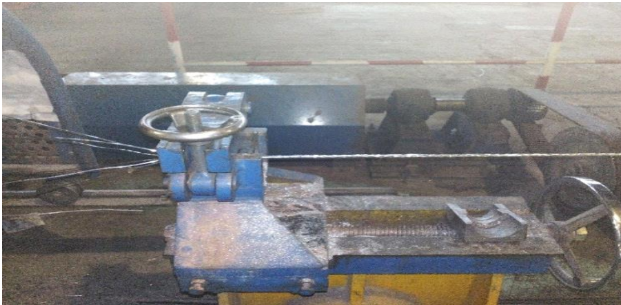
Figure I.6: Processus de câblage
