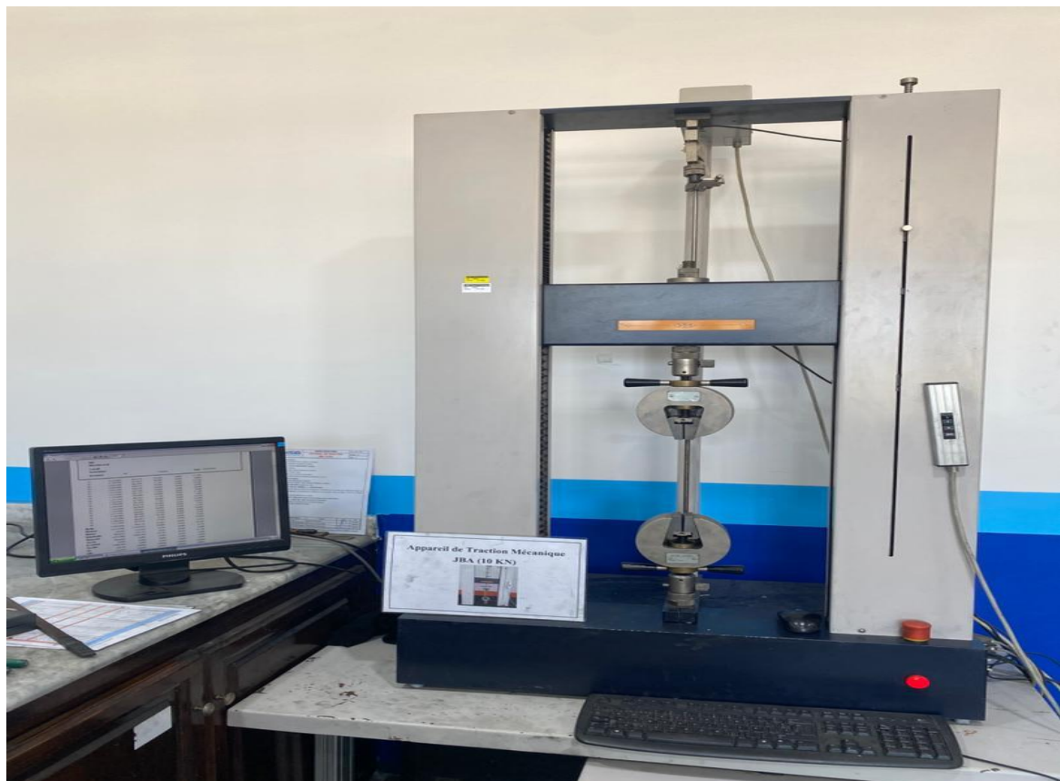
Figure III.16: Appareil de traction mécanique JBA (10 KN)
