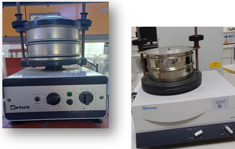
Figure I. 4: Laboratory Siever used during the preparation of the activated carbons ( Retsch )
