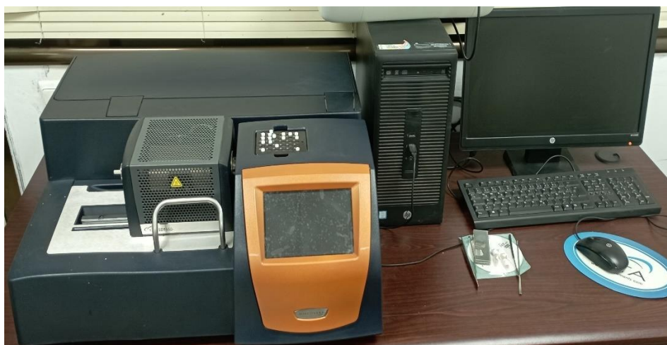
Figure IV.2. 1: Thermogravimetric analyzer Discovery TA-SDT650 used for thermal analysis
