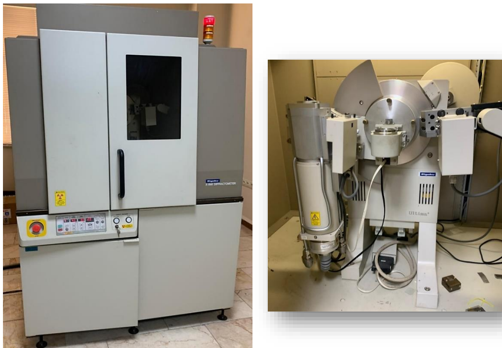
Figure IV. 2. 4: X-ray diffractometer (XRD) used for structural analysis
