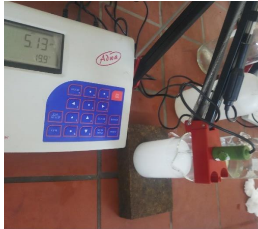
Figure I. 6: pH meter used for pH measurement (ADWA Hungary pH and Conductivity Meter)
