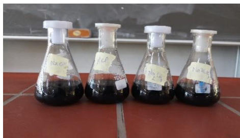
Figure IV.2. 6: Boehm titration procedure
