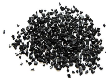
Granular Activated Carbon (GAC):
