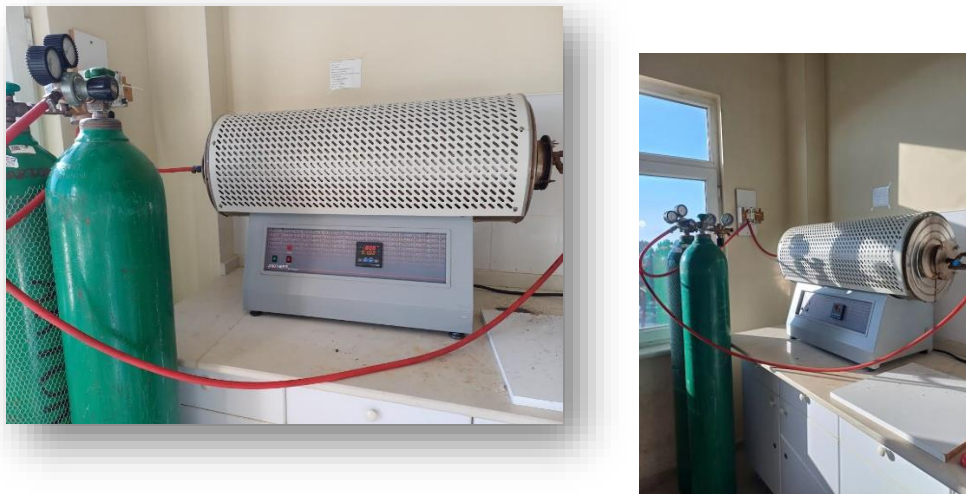
Figure I. 2: Tube furnace used under nitrogen atmosphere (Protherm furanace)
