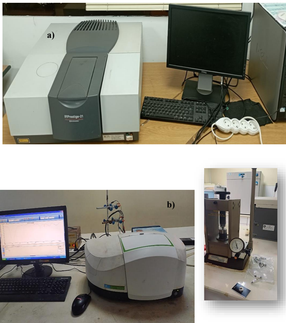
Figure IV 2. 5: FT-IR spectrometers used for functional group identification, a) Prestige-21 SHIMADZU spectrophotometer, b) Perkin Elmer Spectrum Two spectrophotometer.
