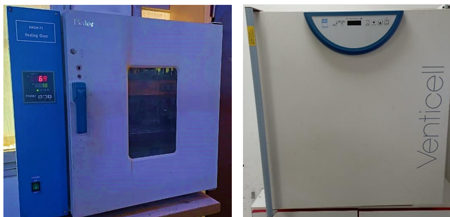
Figure I. 5: Drying oven used in the Laboratory (HRDH-71 and venticell)
