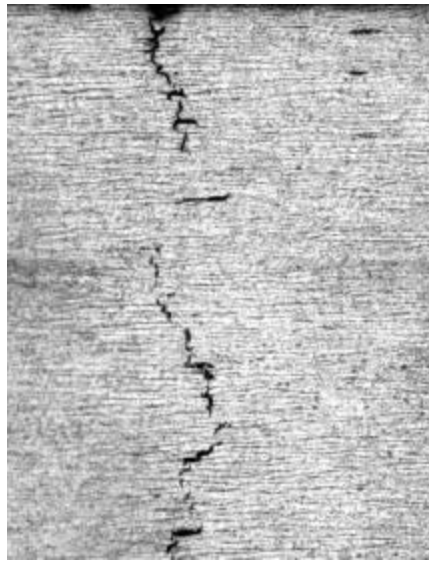
Figure III-6 : Fissuration de type SOHIC [45].
