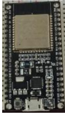
Figure II-3: ESP32 development board used as the main controller
