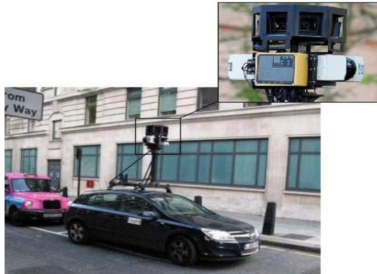
Figure II.12: Acquisition des photos de façades
