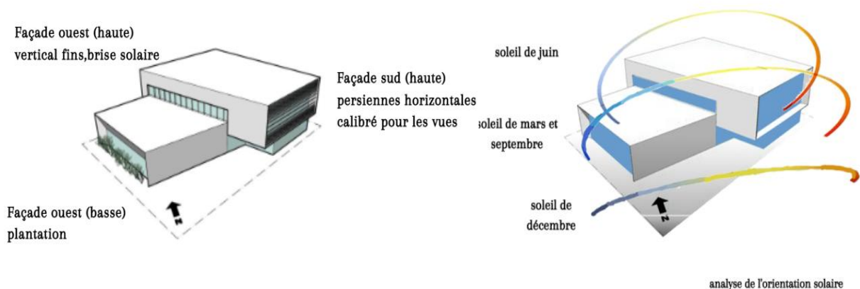
Figure 37: Façade bioclimatique (Source: Marble Fairbanks Architects, Archidaily ,2020)
