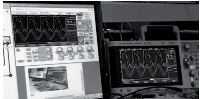
Fig. 6. Real and remote distance panel of an oscilloscope.
