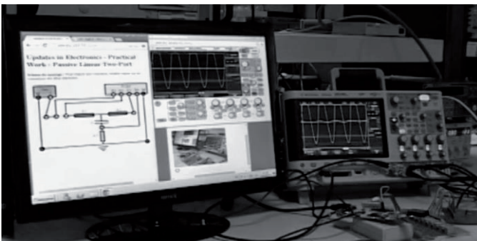
Fig. 5. Experimental real lab remote interface.
