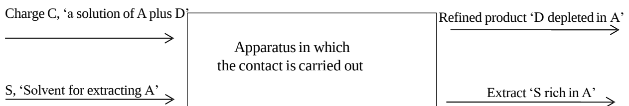
Fig. II.1. Schematic diagram of a liquid-liquid extraction process.
