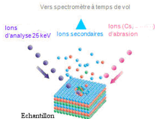
Figure III.6 : Principe du ToF-SIMS
